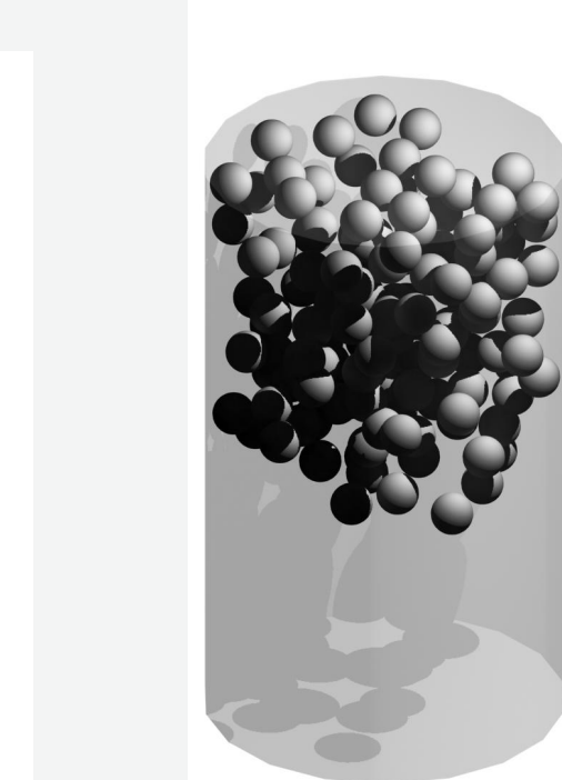
Spherical PCM Pellets work directly in the hydraulic fluid
